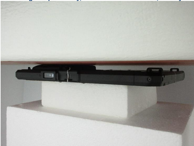
Testing Setup for Body, Bottom Surface at 0 mm, Battery1
