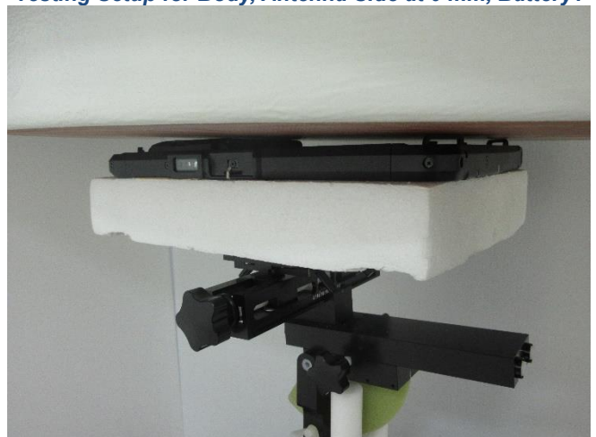
Testing Setup for Body, Antenna Side at 0 mm, Battery1
