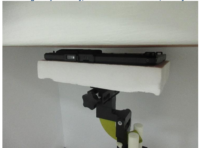
Testing Setup for Body, Bottom Surface at 4 mm, Battery1
