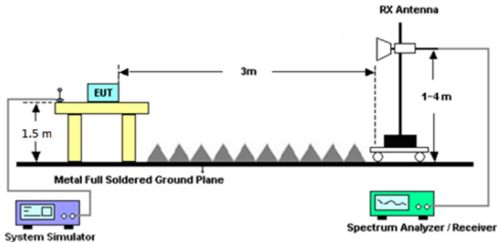
For radiated test above 18GHz
