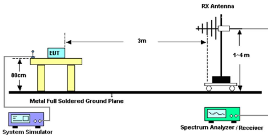
For radiated test from 1GHz to 18GHz
