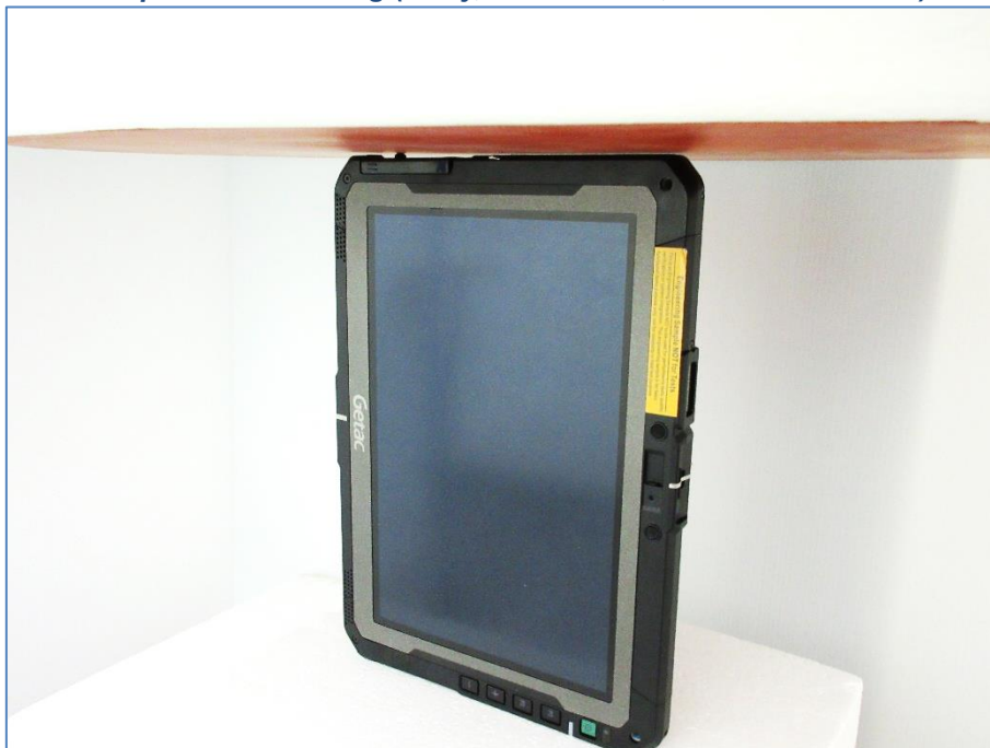
Setup for SAR Testing (Body, Tablet mode, Left Side at 0 mm)
