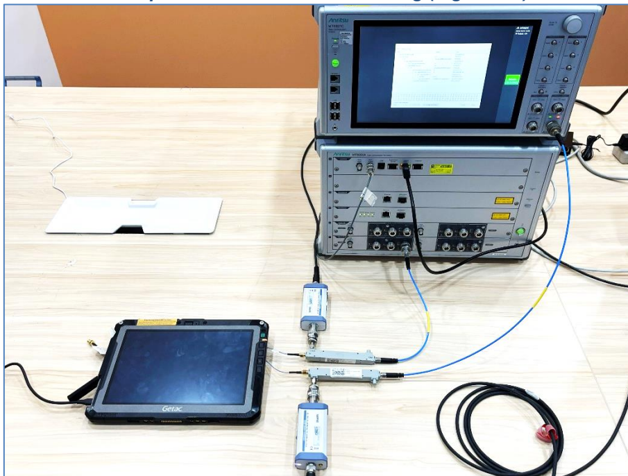
Setup for Conducted Power Testing (Figure 4-6)
