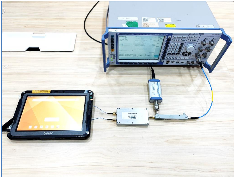
Setup for Conducted Power Testing (Figure 4-5)
