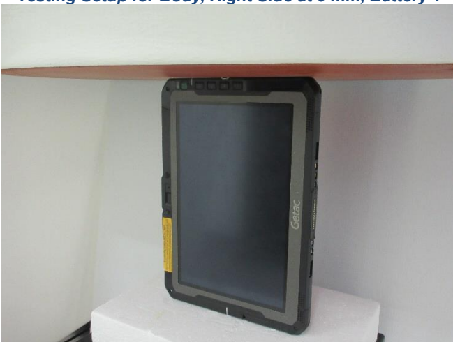
Testing Setup for Body, Right Side at 0 mm, Battery 1
