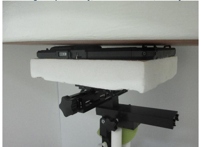
Testing Setup for Body, Ant Side at 0 mm, Battery 1
