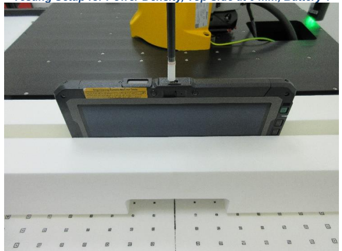
Testing Setup for Power Density, Top Side at 0 mm, Battery 1
