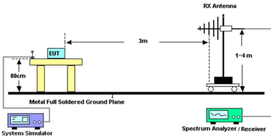
For radiated test from 1GHz to 18GHz
