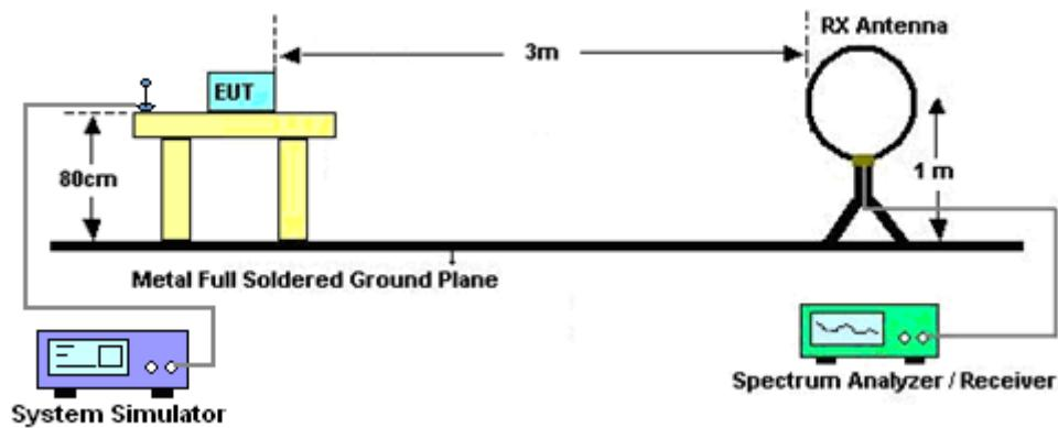
For radiated test from 30MHz to 1GHz
