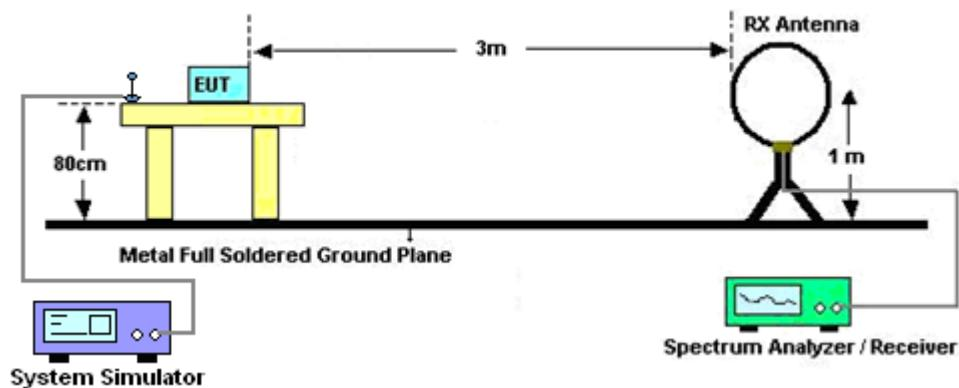
For radiated emissions from 30MHz to 1GHz
