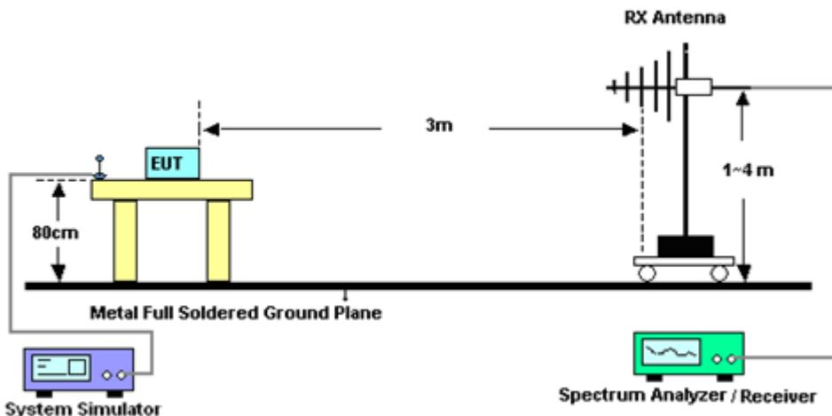
For radiated emissions from 1GHz to 18GHz
