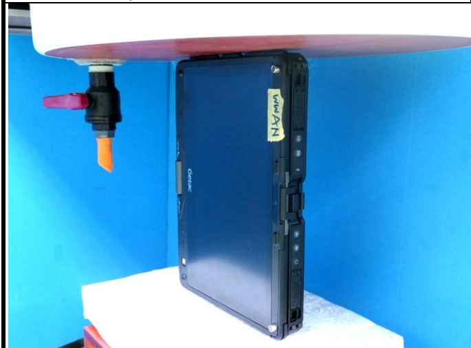
Body - Left Side of EUT at 0 mm
