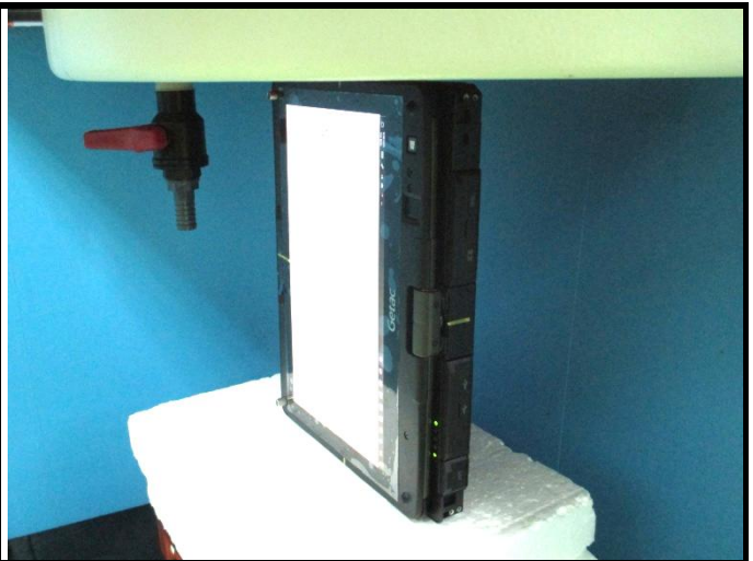
Body - Right Side of EUT at 0 mm
