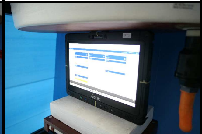
Top Side of EUT with Battery1 Tested at 0 mm
