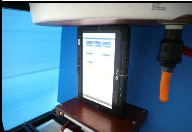
Right Side of EUT with Battery1 Tested at 0 mm
