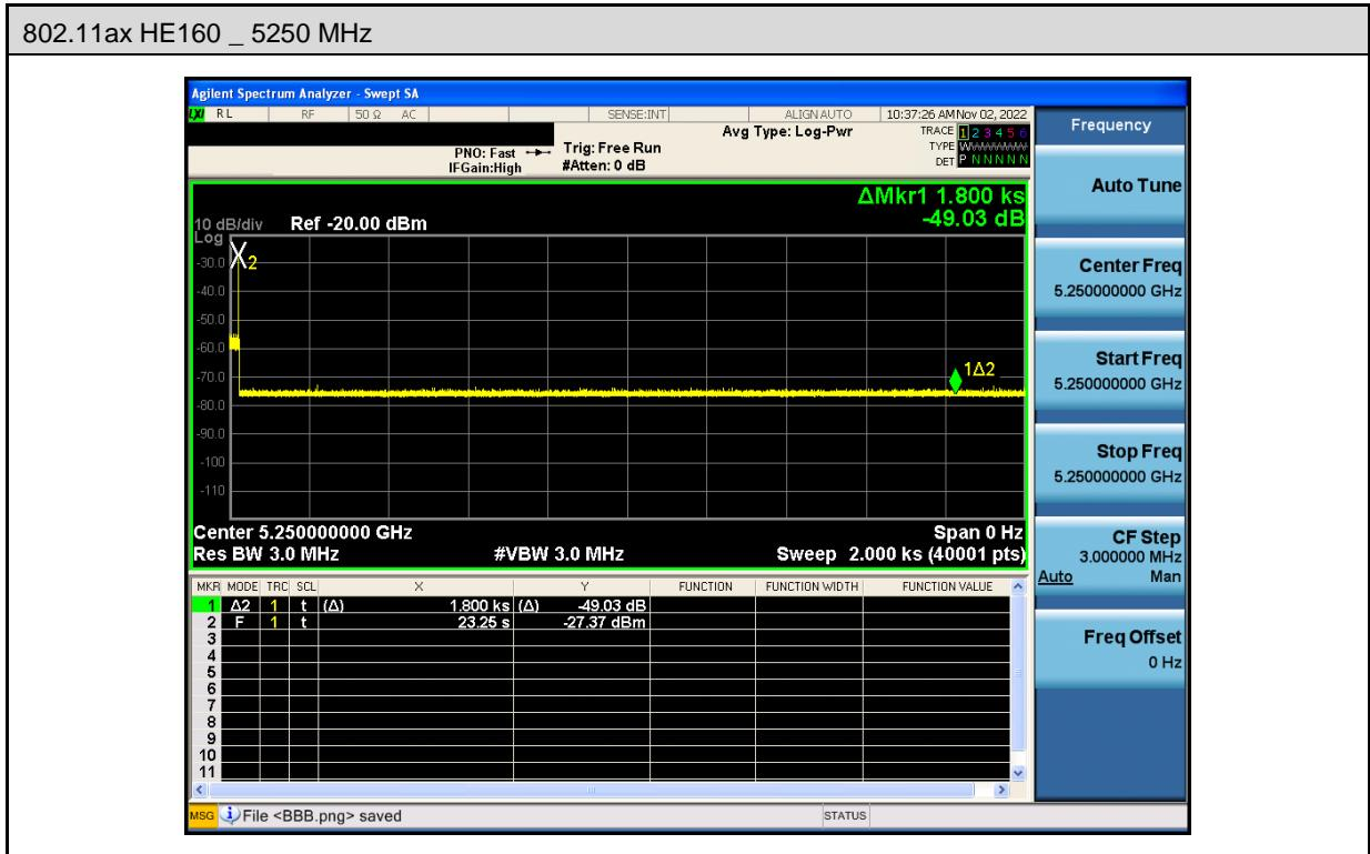
Note: Non-Occupancy Period time is 30 minute during which a Channel will not be utilized after a Radar Waveform is detected on that Channel.
