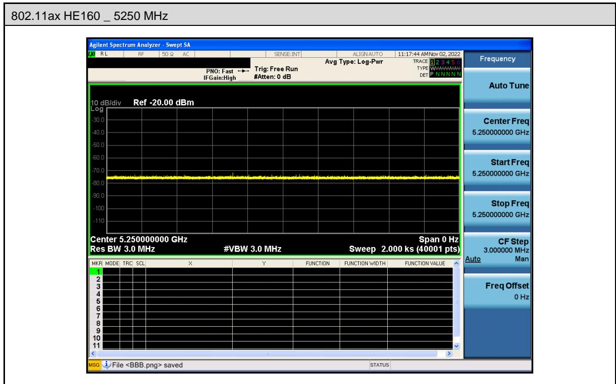
Note: The non-associated Client Beacon Test is during the 30 minutes observation time. The EUT should not make any transmissions in the DFS band after EUT power up.
