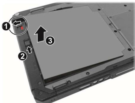
3. Fit another battery pack into place. With the battery pack correctly oriented, attach its connector side to the battery compartment at an angle (1) and then press down the other side (2). The battery release latch should automatically engage.
