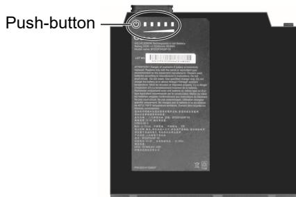
When the battery pack is not installed in the Tablet PC and you want to know the battery charge, you can press the push-button to see the number of LEDs that light up. Each LED represents 20% charge.
