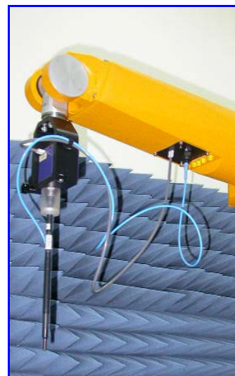
Figure 2. Probe setup on robot
