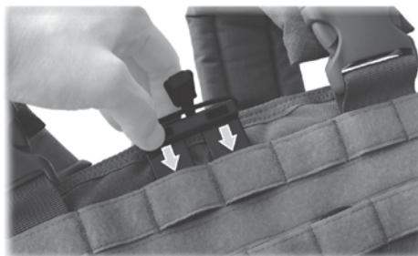
4. Align the bottom grooves of MX50 with the counterparts on the mount and insert MX50 at an angle (1). Then press the holder and MX50 together until the clamp clicks into place (2).
