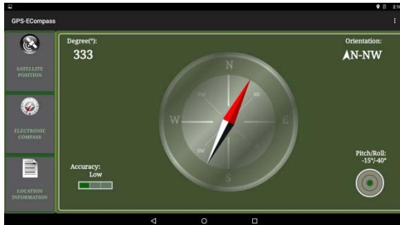
The Accuracy reading is for your reference. When the application determines that calibration is needed, it will pop up the “Calibration” graphics asking you to calibrate the compass. Hold the device and swing it in the way as shown on the screen. Do this several times until the popup graphics disappear.
