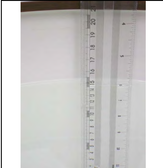
Figure 6. Liquid Height for Body SAR
