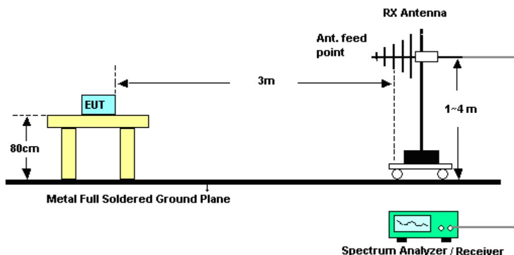
**For radiated emissions above 1GHz**
