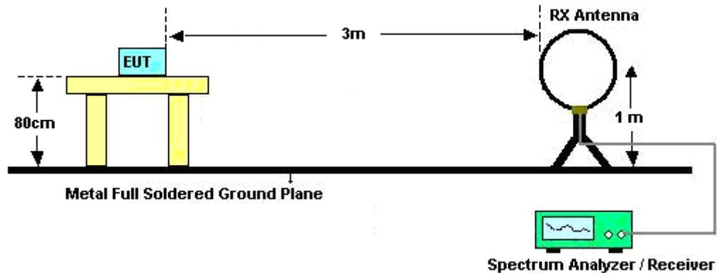
For radiated emissions from 30MHz to 1GHz
