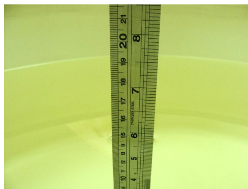
Fig 6.2 Photo of Liquid Height for Body SAR
