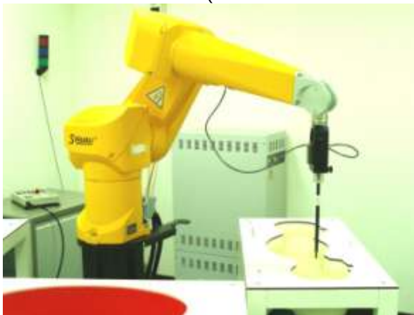
Fig 5.5 Photo of DASY4
