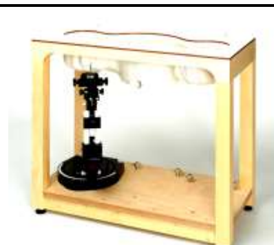
Fig 5.9 Photo of SAM Phantom
