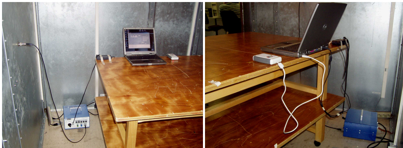
Conducted emission test setup
