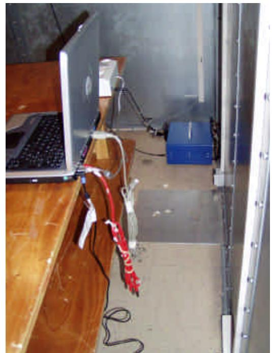
The EUT is placed on a table at 0.8m height. The EUT (LDB307 & AC/DC converter) is powered through the LISN (measured). The peripheral equipment (PC) is connected to a separate LISN.
