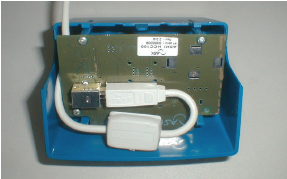
HCC 100 docking station (Lower part of plastic housing removed)
