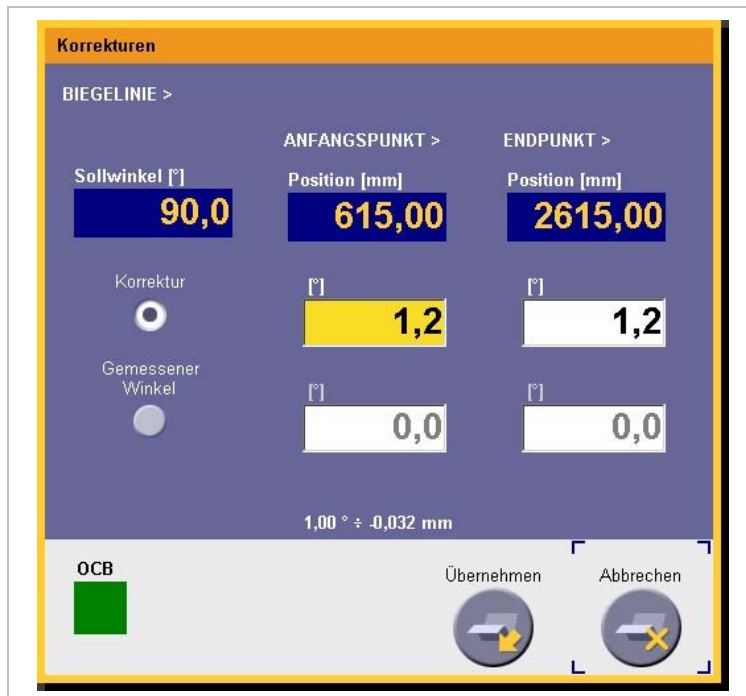
Transfer of the measured angle
