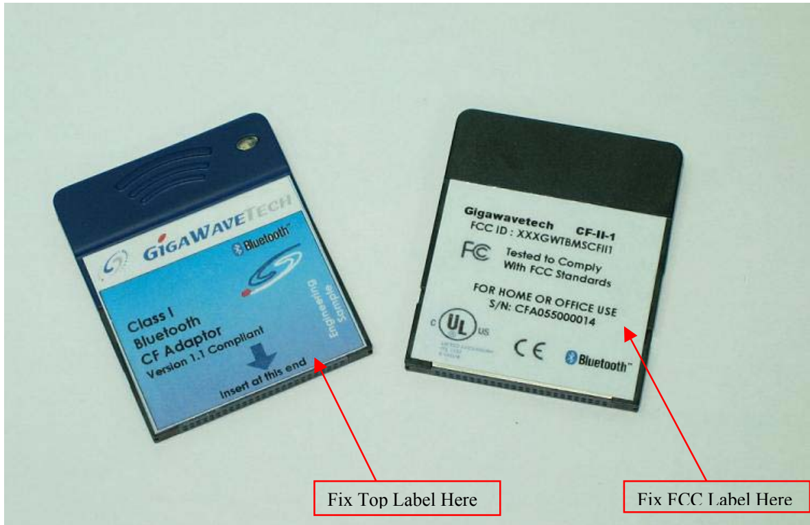
Illustration of the fixing of the Front and FCC Label on the CF Card
