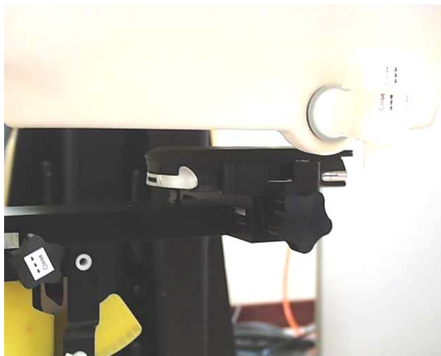
SAR Test Setup At Flat Phantom – Closer View (EUT Rear To Phantom, 15mm spacing)
