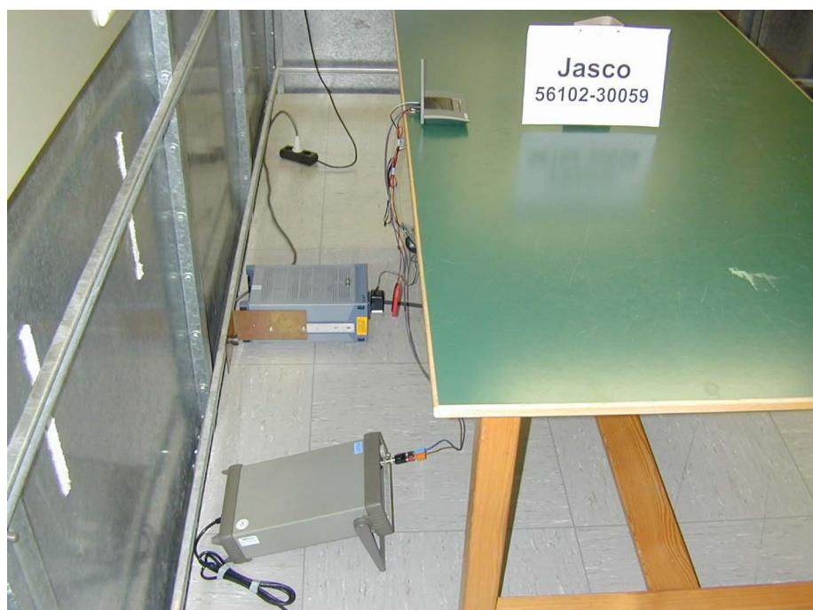
**Test setup for radiated emission measurement**
