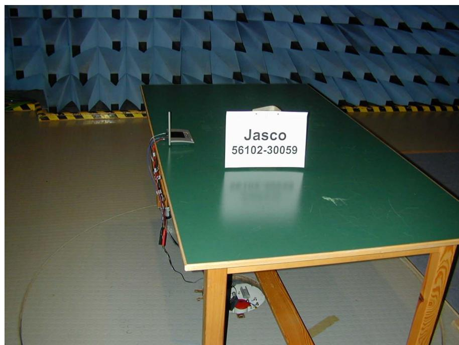
**Test setup for radiated emission measurement**
