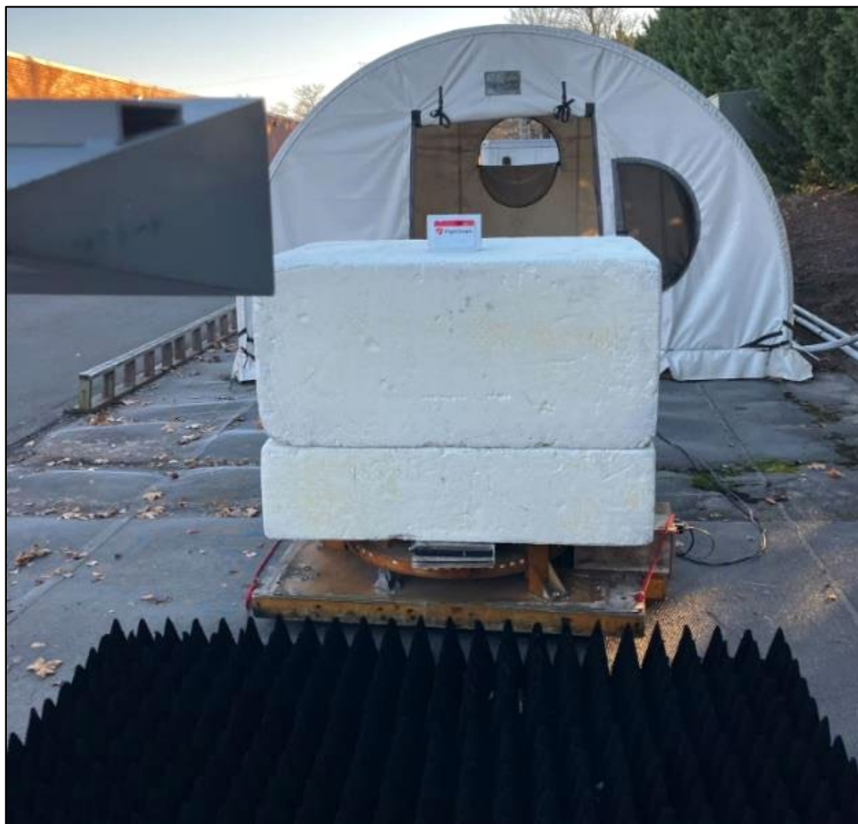
Photograph 4: Radiated Emissions Testing – Front View (Above 1 GHz)
