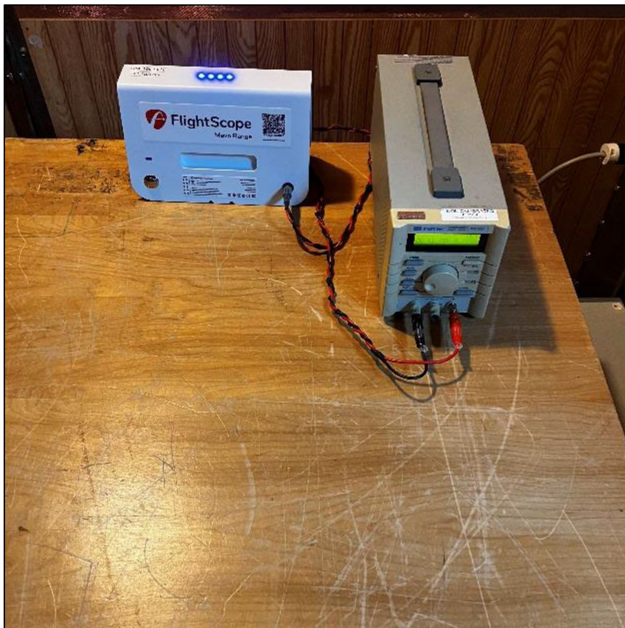
Photograph 6: AC Conducted Emissions Testing – Front View
