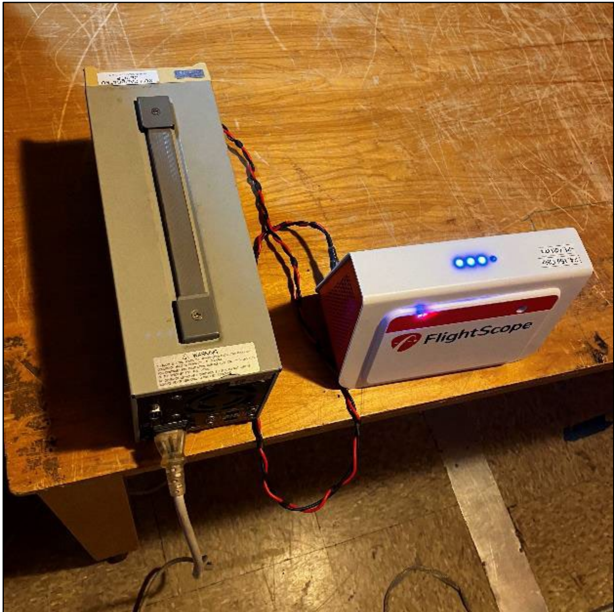
Photograph 7: AC Conducted Emissions Testing – Rear View
