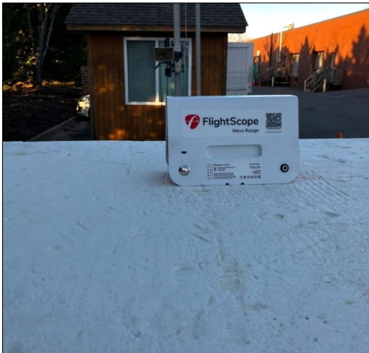
Photograph 5: Radiated Emissions Testing – Rear View (Above 1 GHz)
