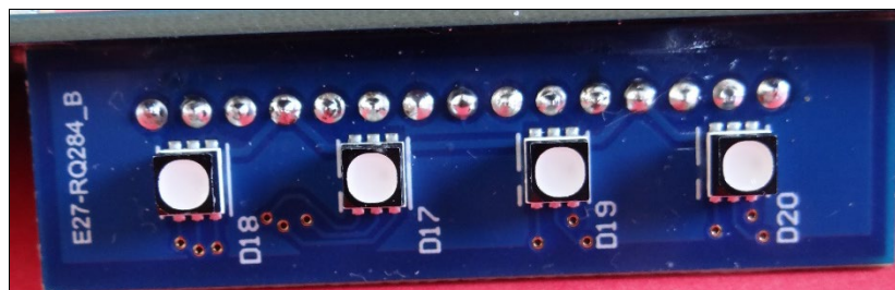
Top View of LED PCB fitted to FS MEVO Range PSU &amp; Charger PCB
