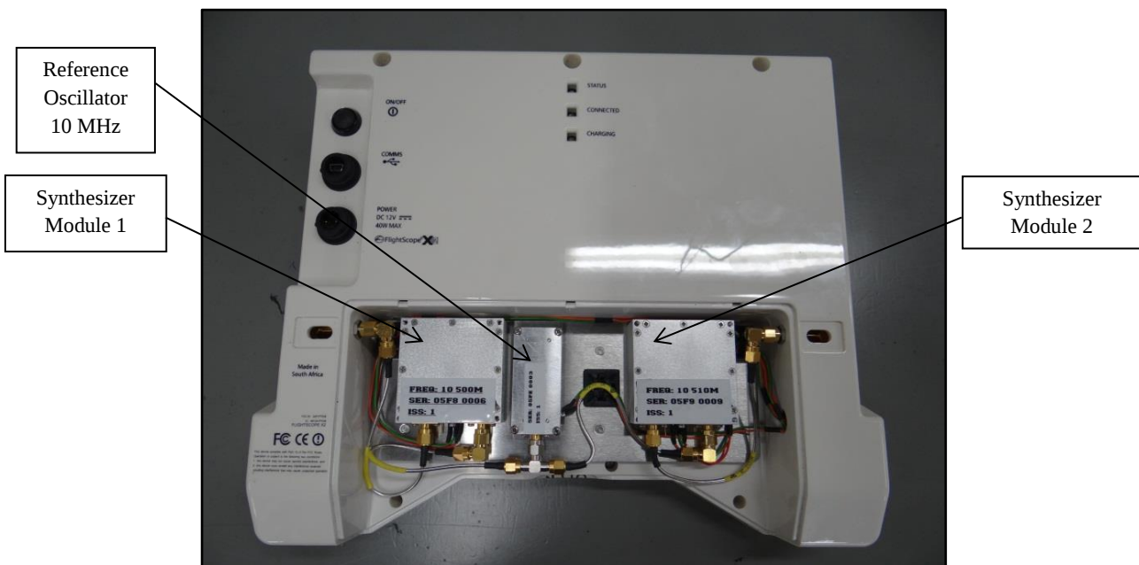
Rear Equipment View with cover removed
