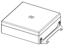
Figure 2 AP5050U flat surface installation with metal “L” brackets
