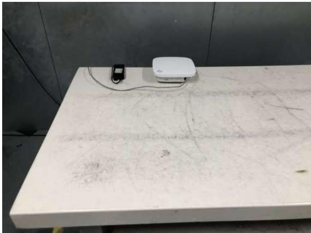
Description: Conducted emission Test Setup(AP460C)
