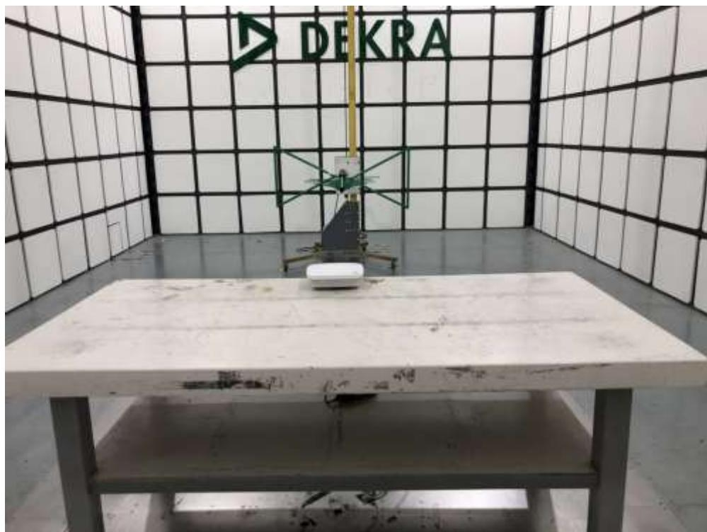
Description: Radiated Emission Test Setup for 1~18GHz(AP460C)
