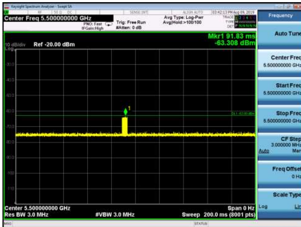
11a CH100 5500MHz Radar Type 2 Calibration Plot
