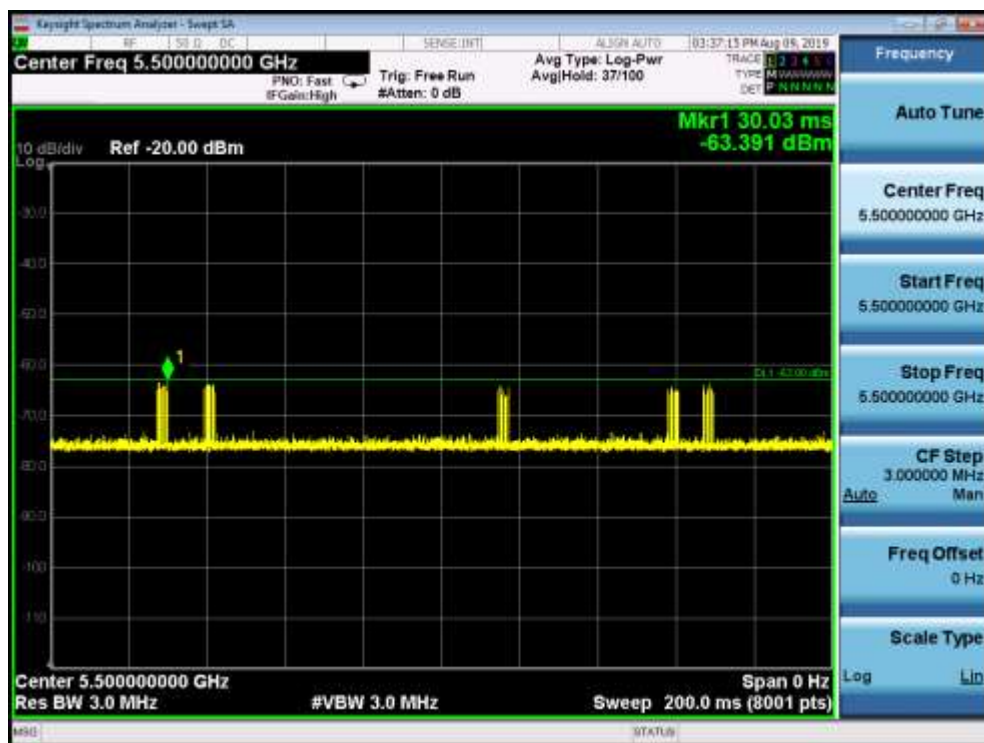
11a CH100 5500MHz Radar Type 6 Calibration Plot
