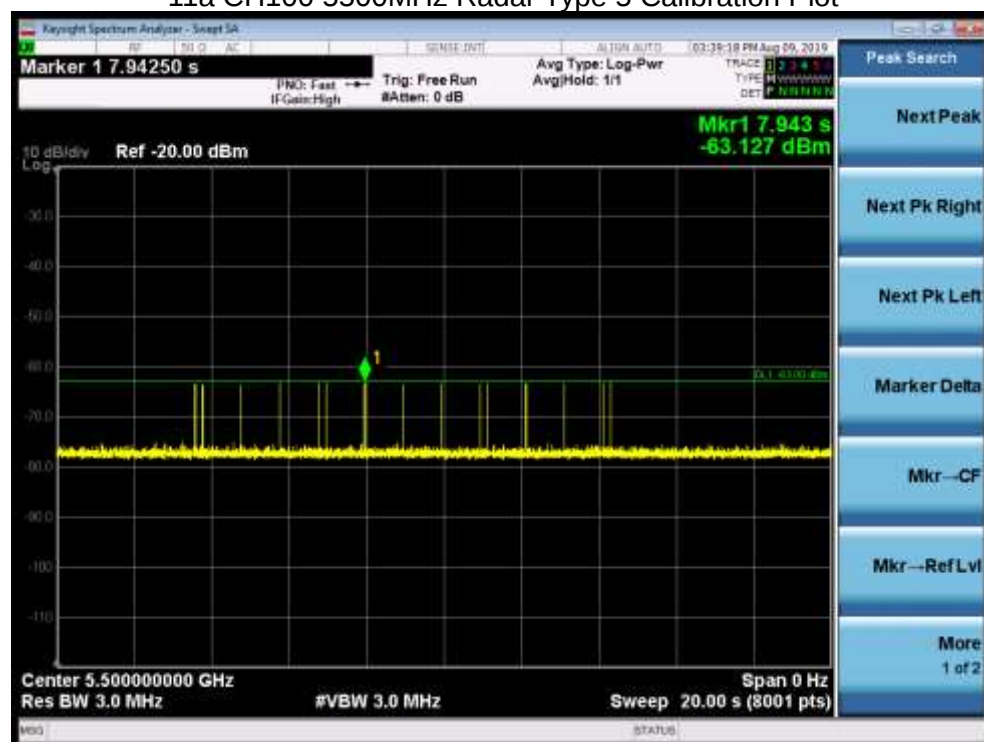
11a CH100 5500MHz Radar Type 5 Calibration Plot
