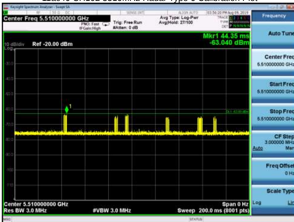
11ac40 CH102 5510MHz Radar Type 6 Calibration Plot
