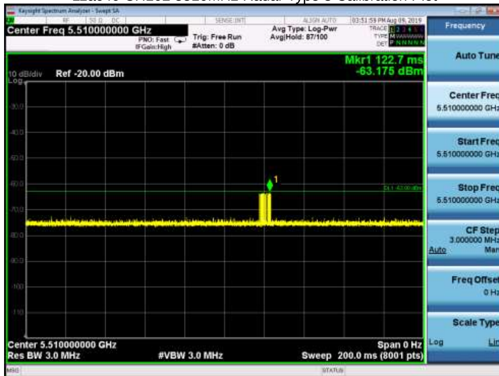
11ac40 CH102 5510MHz Radar Type 3 Calibration Plot
