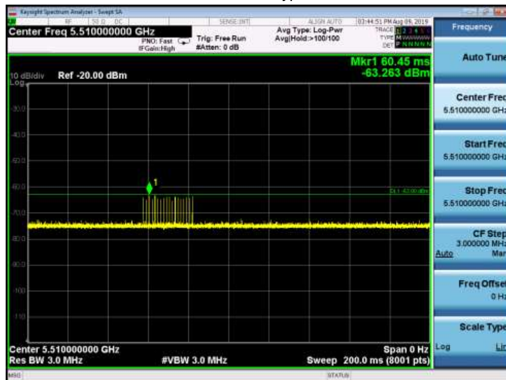
11ac40 CH102 5510MHz Radar Type 0 Calibration Plot
