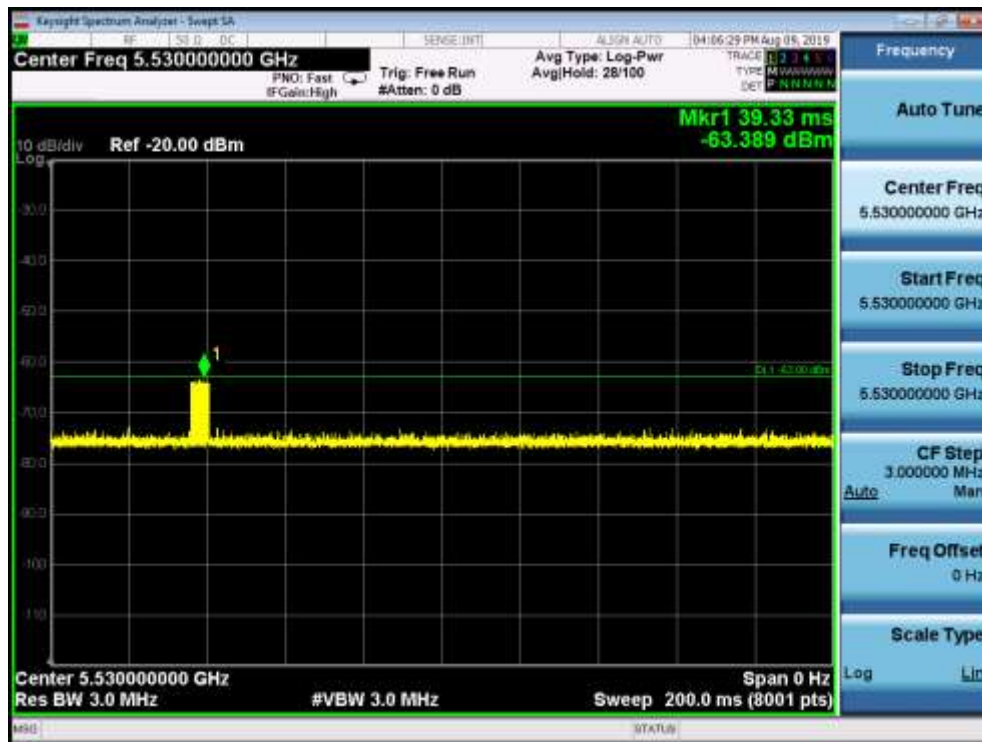
11ac80 CH106 5530MHz Radar Type 2 Calibration Plot
