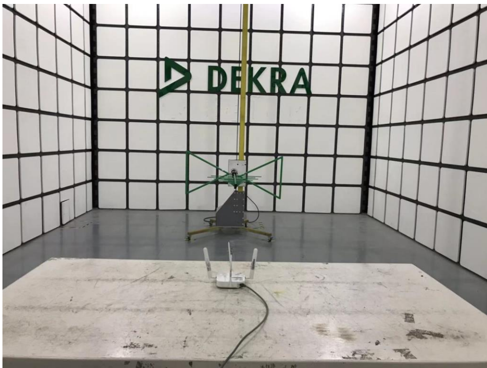
Description: Radiated Emission Test Setup for Below 1GHz(AP305CX)
