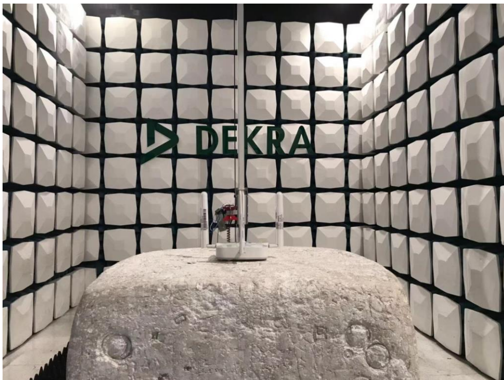
Description: Radiated Emission Test Setup for 1~18GHz(AP305CX)
