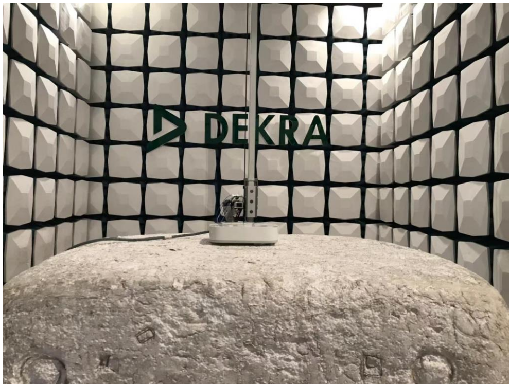
Description: Radiated Emission Test Setup for Above 18GHz(AP305C)
