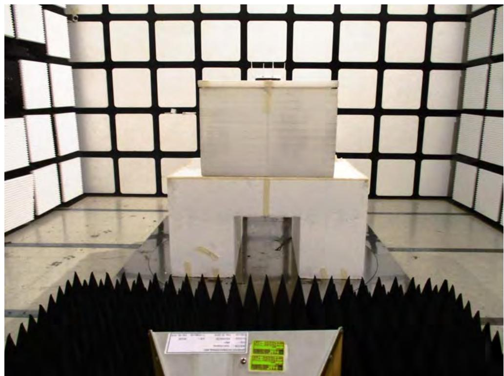
**Test Mode 8: EUT 2 + Set 10 PIFA Antenna / Chain1:5.84 dBi, Chain2:5.50 dBi, Chain3:5.84 dBi, Chain4:5.65 dBi**
