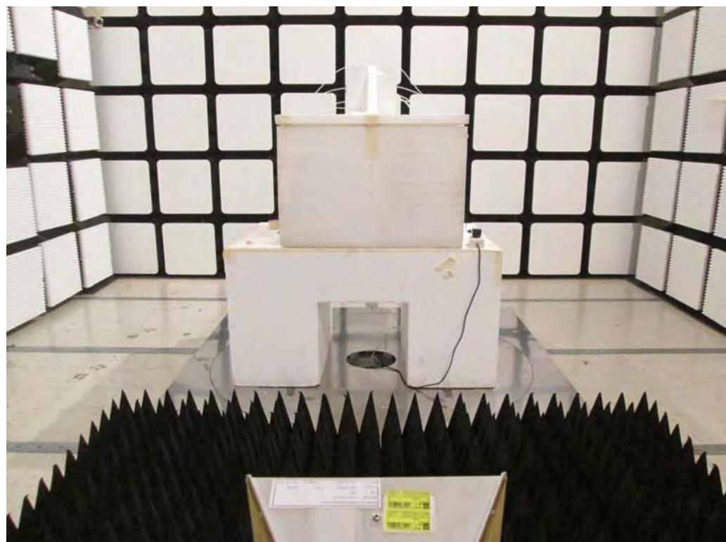
**Test Mode 3: EUT 1 + Set 3 Sector Antenna / 5.5 dBi**
