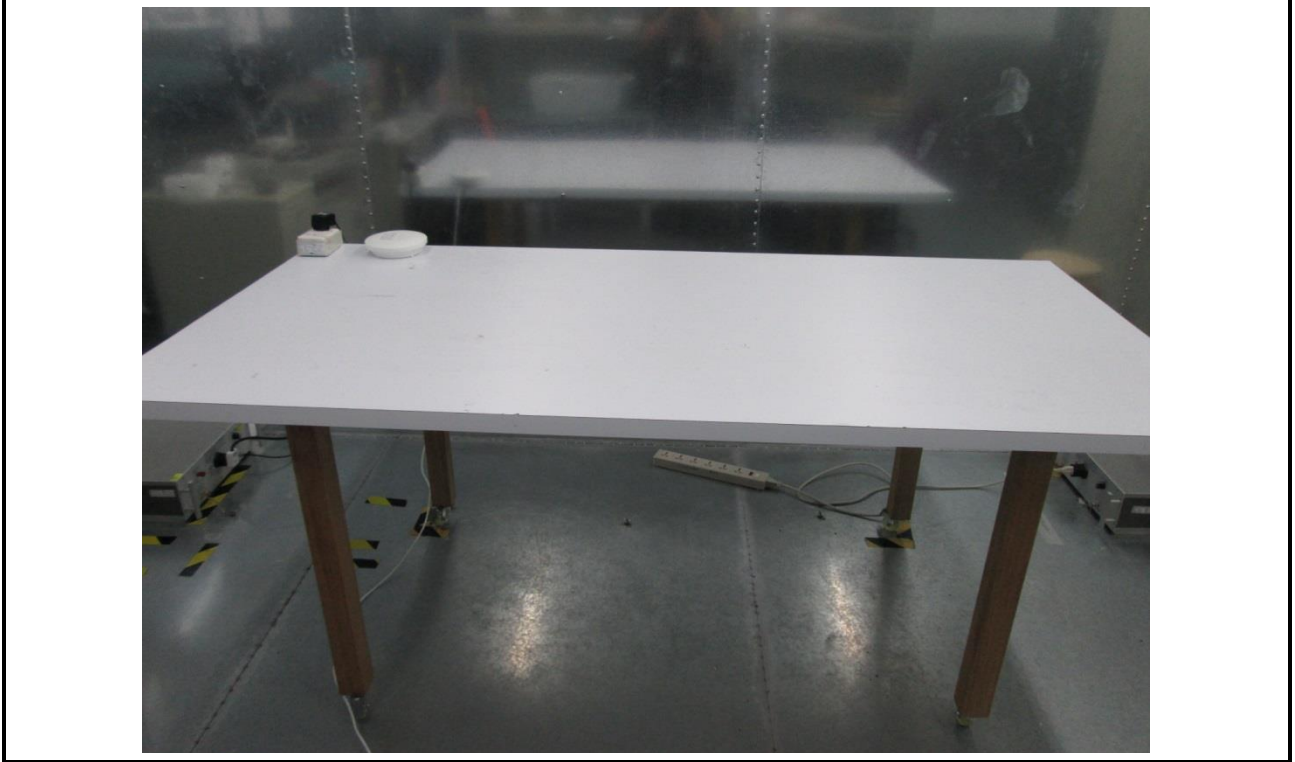
Conducted Emission Test (PIFA antenna, Adapter mode)
