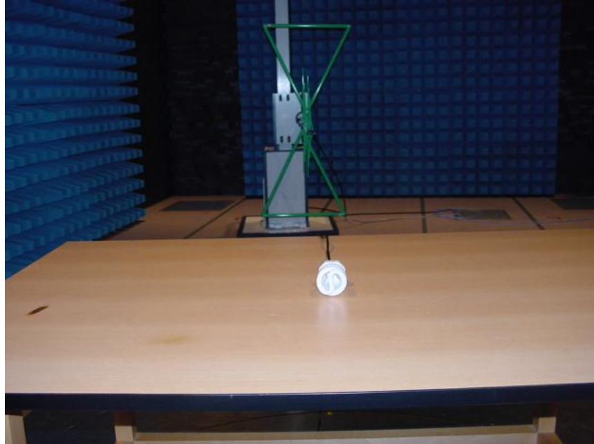
Radiated emission test view for EUT series
