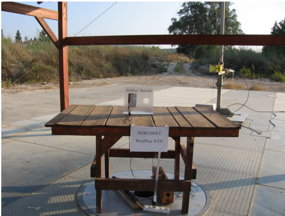
Figure 7. Radiated Emission Test Front
