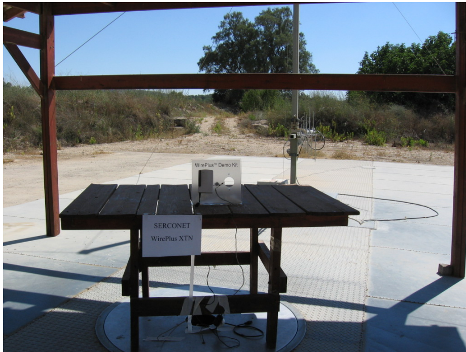
Figure 6. Radiated Emission Test Front
