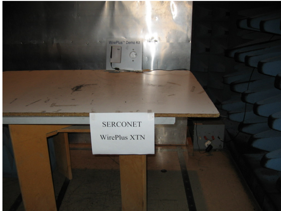
Figure 4. Conducted Emission From AC Mains Test Front
