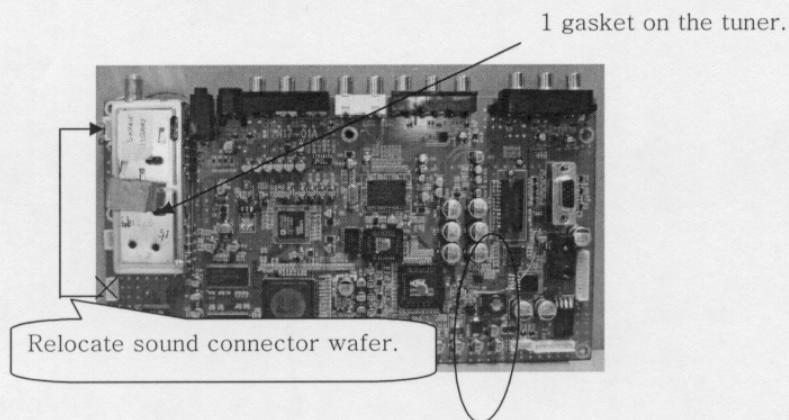
3. Relocate the connector wafer which outputs TV sound and its additional works.
