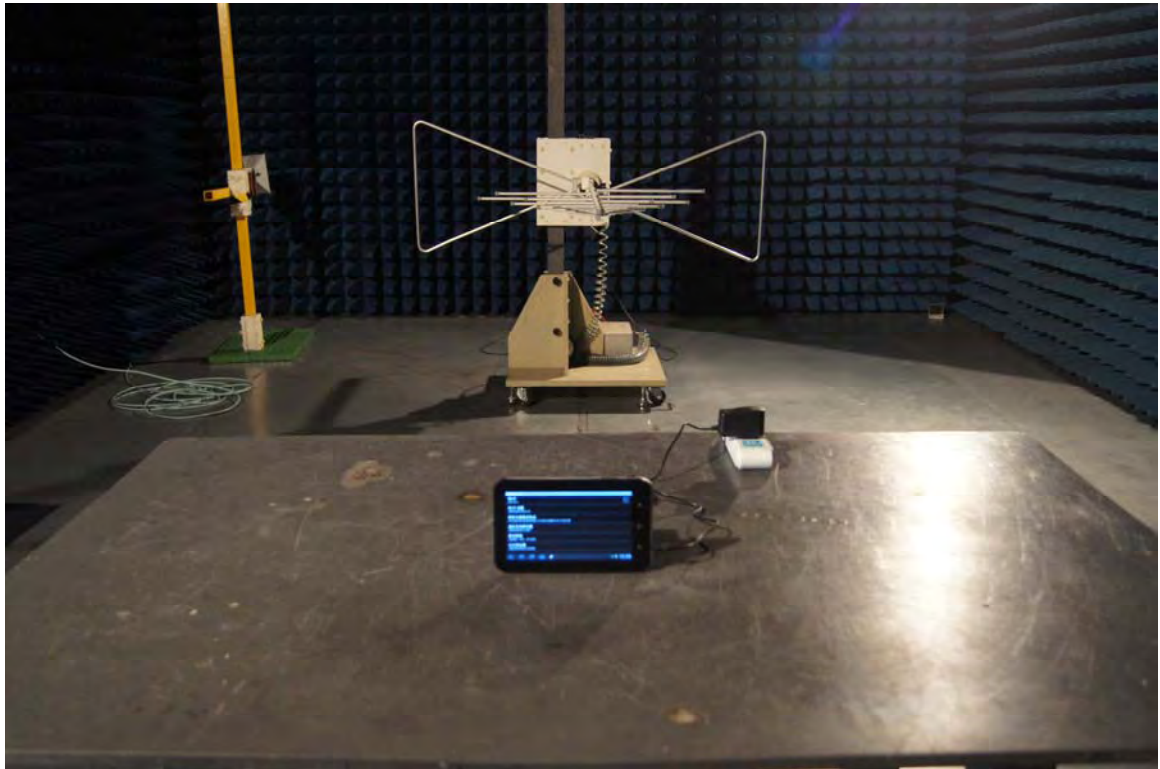
Radiated emissions test 30MHz- 1GHz (Part 15C)
