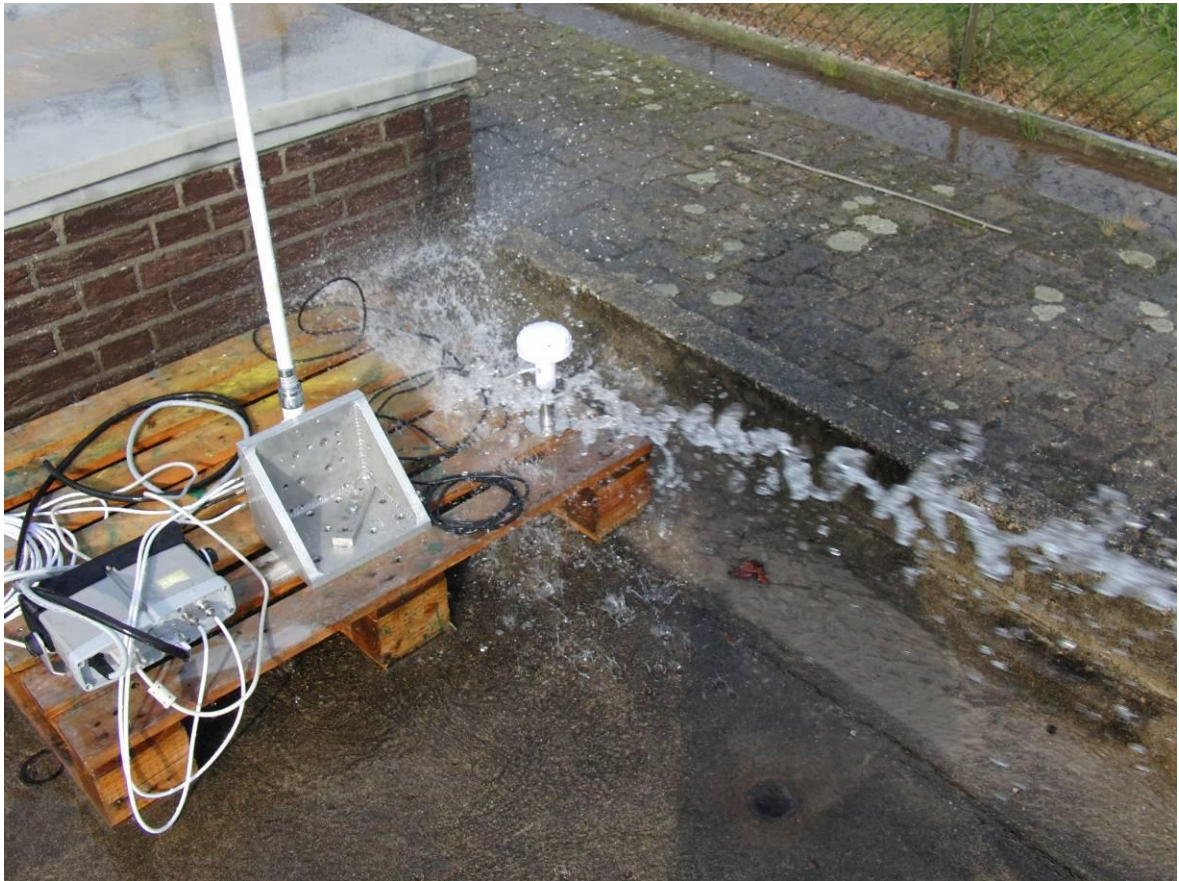
Photograph 18: Spray test on MA-700
