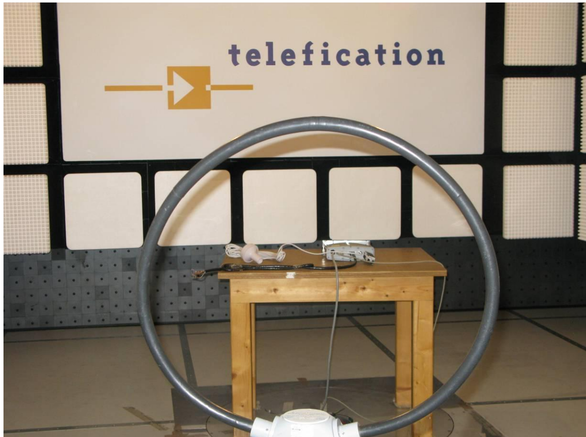
Photograph 9: radiated emissions test set up (0.15 – 30 MHz)
