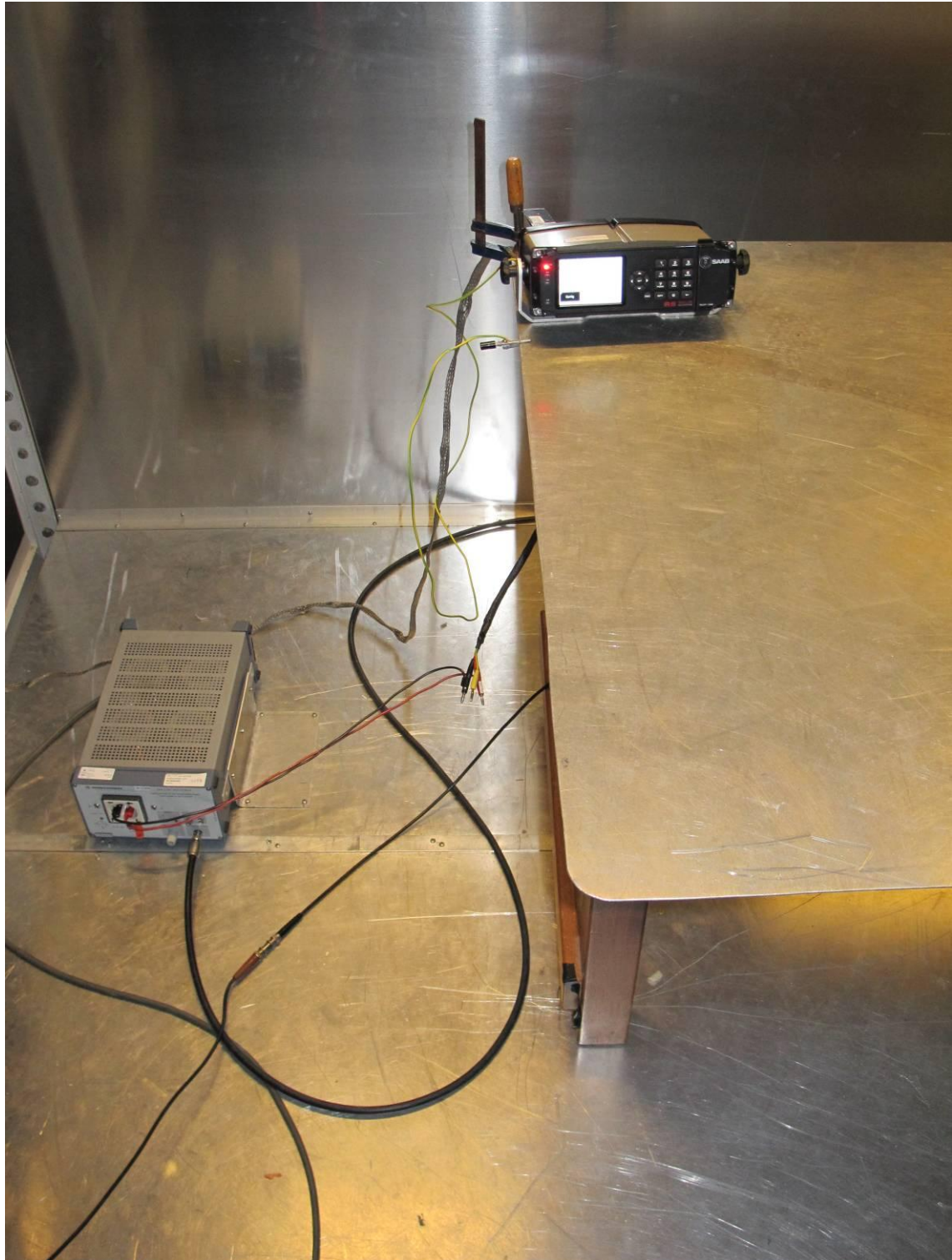
Photograph 8: conducted emissions test set up (0.01 – 30 MHz)
