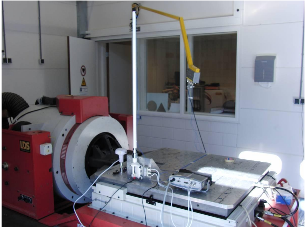
Photograph 12: Vibration test setup with R5 in original bracket mount (1 st horizontal direction)
