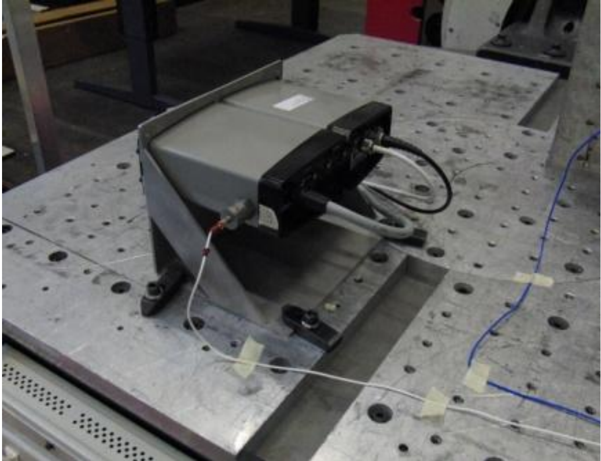
Photograph 17: Vibration test setup with R5 in flush mount (2nd horizontal direction)
