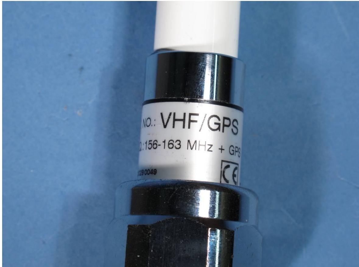
Photograph 7: antenna type VHF/GPS labeling
