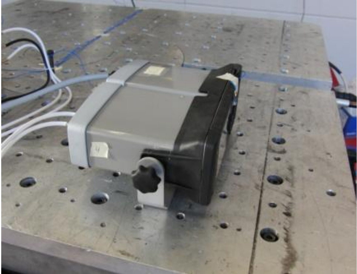
Photograph 14: Vibration test setup with R5 in original bracket mount (2nd horizontal direction)
