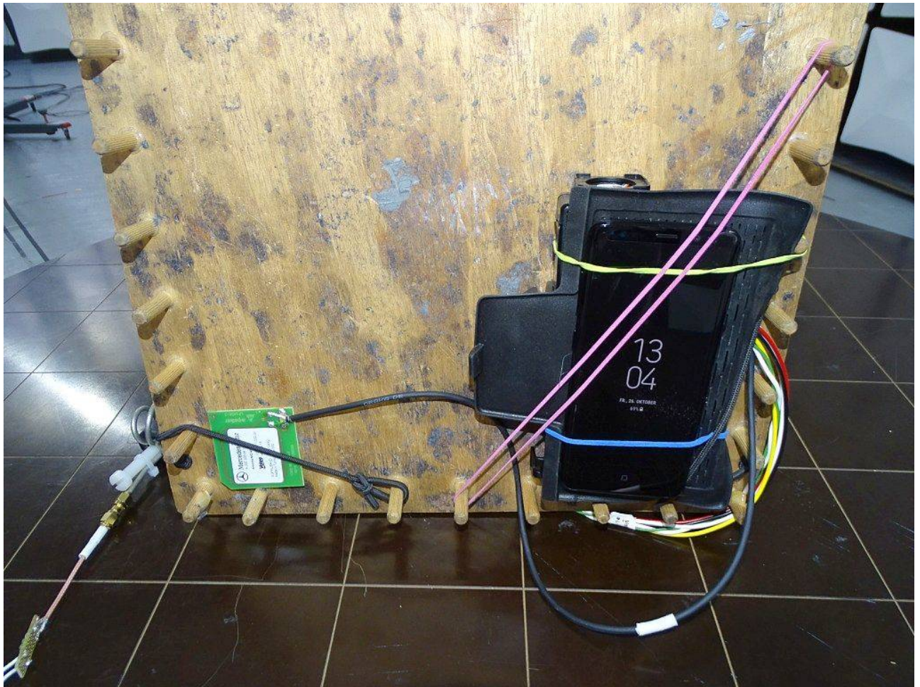
Photo 6: Test setup for radiated measurements (Enclosure, semi-anechoic chamber, NFC integral antenna, detail)
