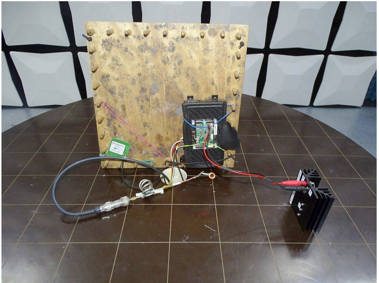
Photo 2: Test setup for radiated measurements (Enclosure, semi-anechoic chamber, 9 kHz to 30 MHz, intentional radiator §15, ANSI C63.10) EUT vertical, WPT
