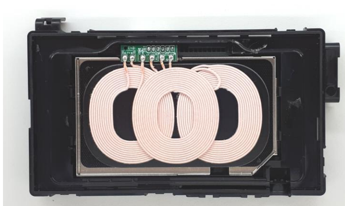
Charging coil element with connector, ferrite plate and metal shield, view from top and bottom side.
