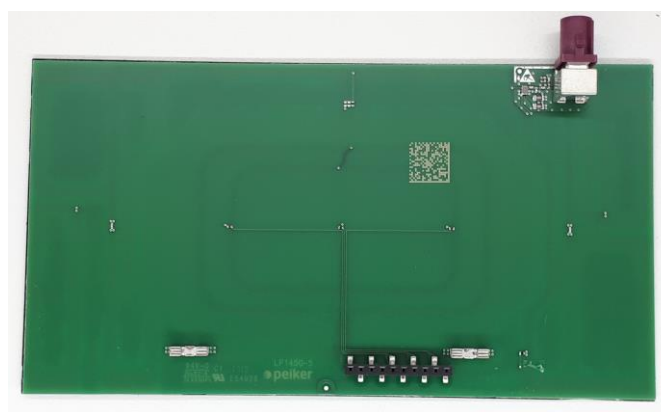
Antenna-PCB (NFC-Antenna and GSM-Coupling-Antenna), top and bottom view. GSM Roof-Antenna and the coupling Antenna (left and right). The NFC-Antenna is in the middle and inner Layer of the PCB.
