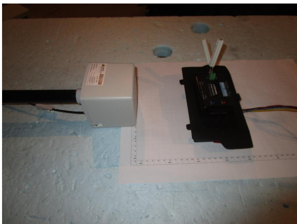
Photograph 8: Measurements in the anechoic chamber, 10cm distance between measurement probe and EUT, Position 3
