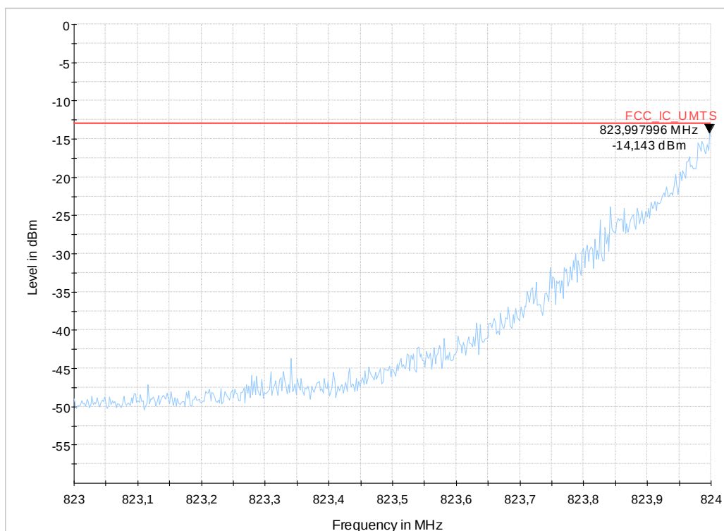
Diagram 9.500a, Channel 20407, QPSK, 1RB low
