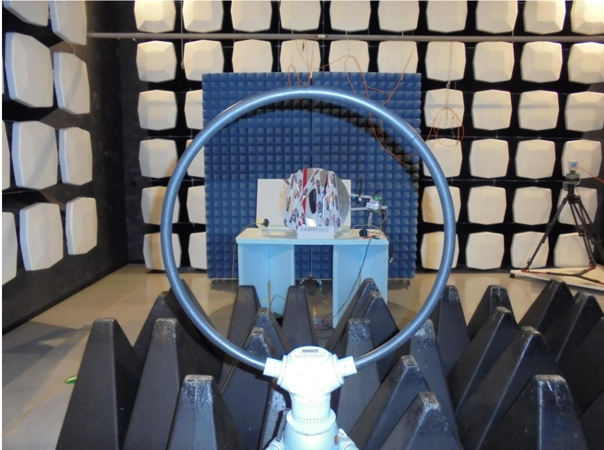
Photograph 7: Measurements in semi-anechoic chamber – Magnetic field
