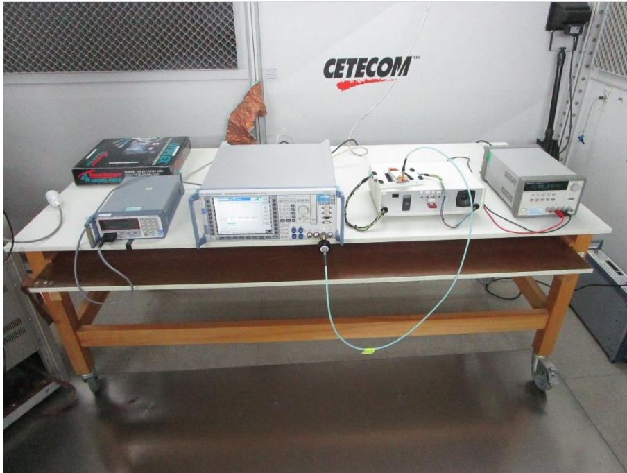
Photograph 7: EUT Setup 3 Conducted RF measurement
