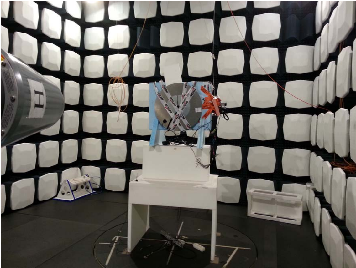
Photograph 1: Measurements in fully anechoic chamber (EUT A in vertical position)
