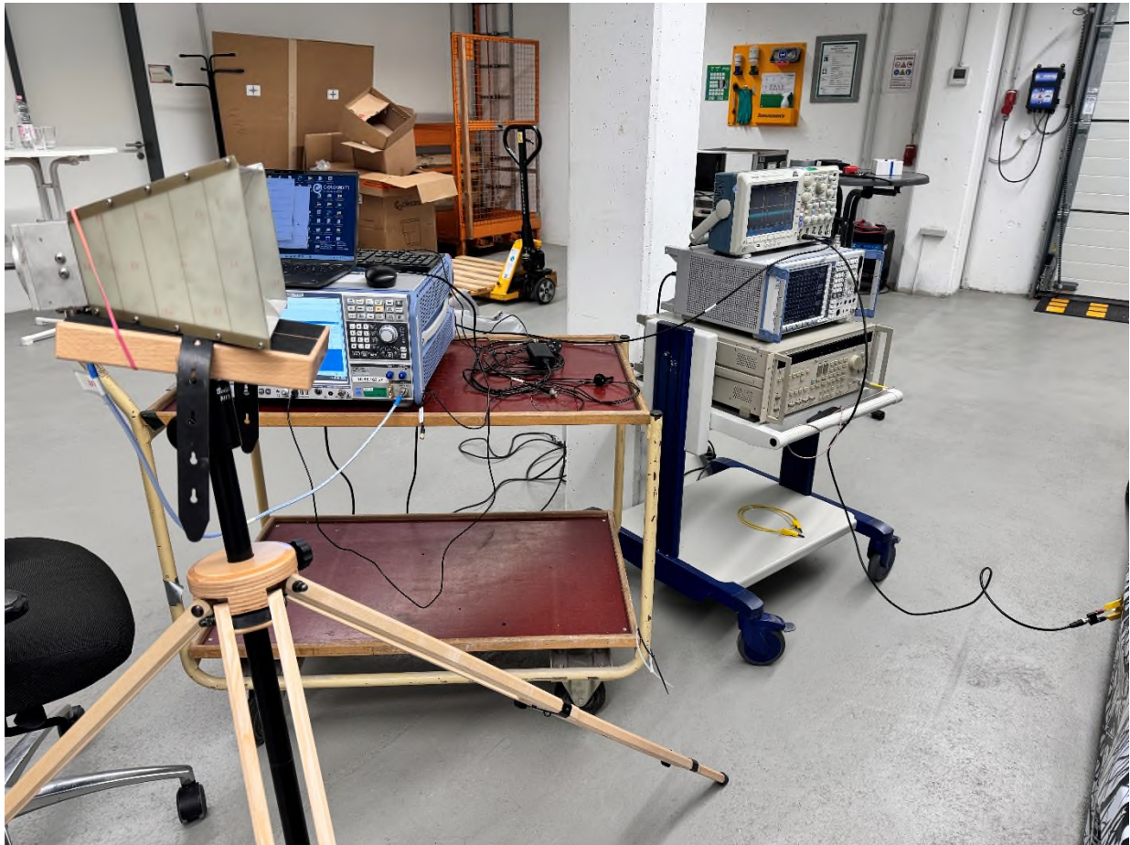
Fig. Mea.: 6 : Radiated RF Parameter Image 6 / Set-up no.3 / Duty-Cycle of transmissions + Timing Part of car (EUT2), only on lower edge right side visible
