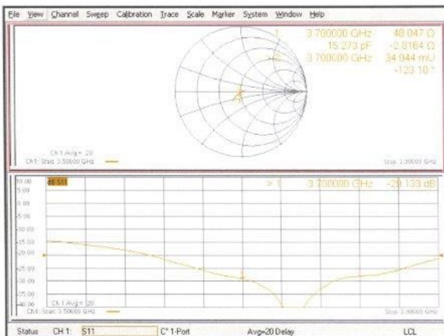
**Antenna Parameters with Head TSL**
