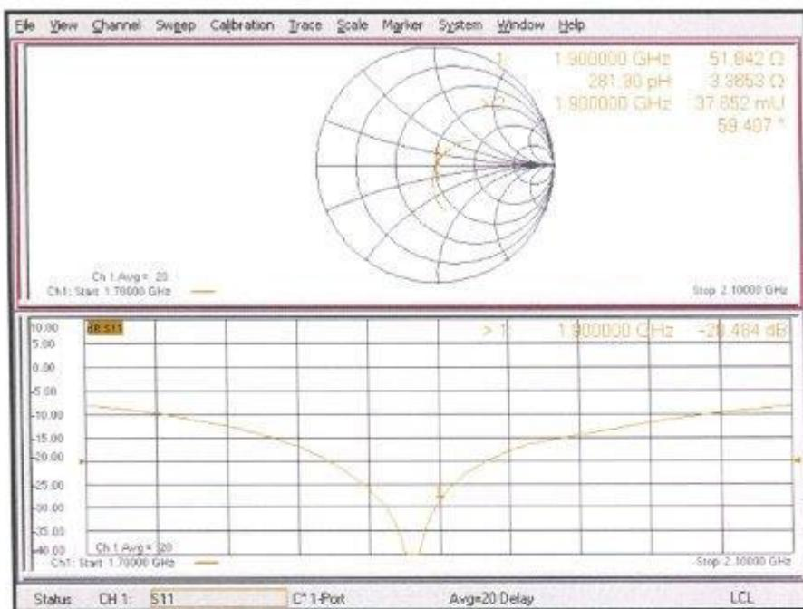
**Antenna Parameters with Head TSL**
