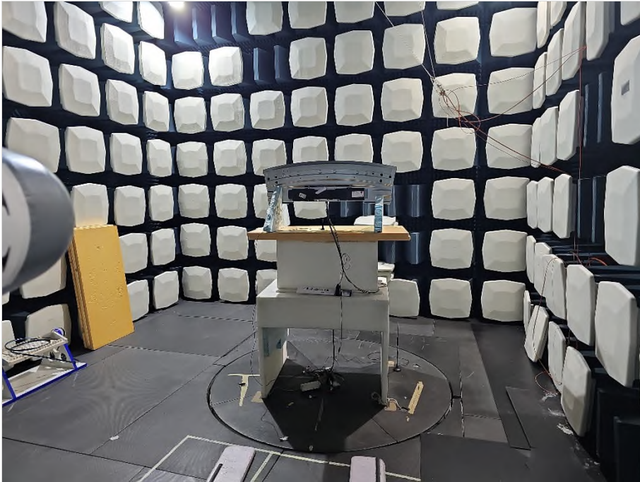
Photograph 7: EUT test setup in the fully anechoic chamber, overview
