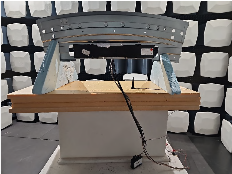
Photograph 6: EUT test setup in the fully anechoic chamber, close up view
