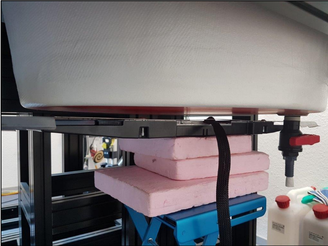
Photo 8: Liquid depth HBBL600-10000MHz Simulating Head Liquid
